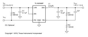
At medium to heavy loads, the device operates in pulse width modulation (PWM) mode with 1.5-MHz switching frequency. At light load, the device automatically enters Power Save Mode (PSM) to maintain high efficiency over the entire load current range. In shutdown, the current consumption is reduced to less than 2 μA.
