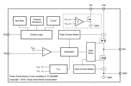
Figure 4. TLV62568 Functional Block Diagram
