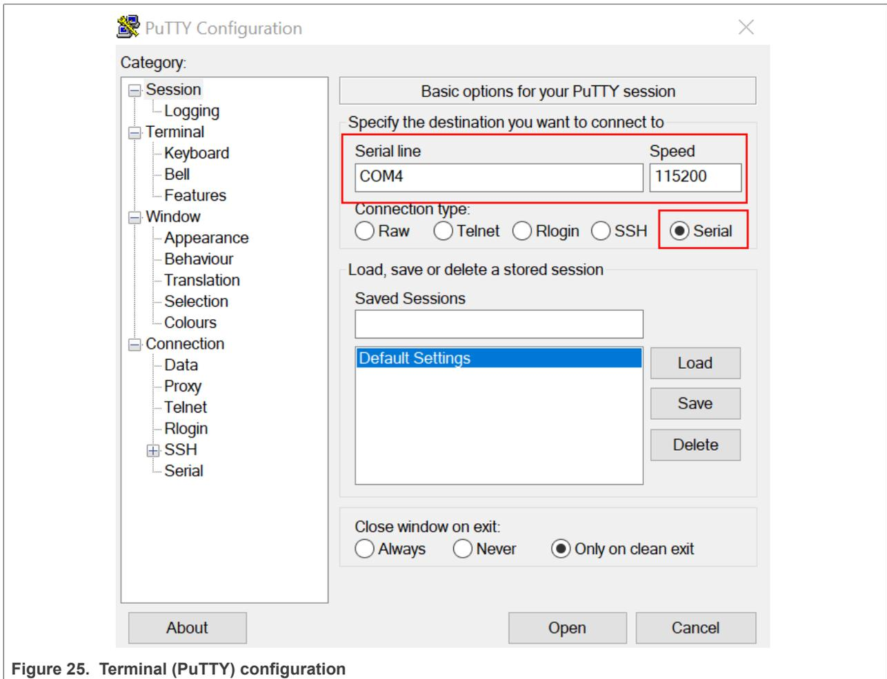
Figure 25. Terminal (PuTTY) configuration
