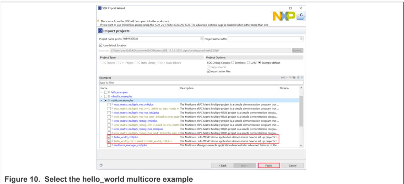
Figure 10. Select the hello\_world multicore example
