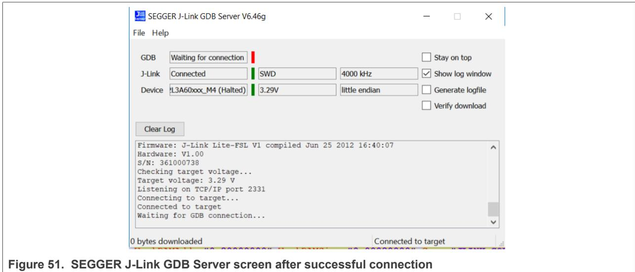
Figure 51. SEGGER J-Link GDB Server screen after successful connection
