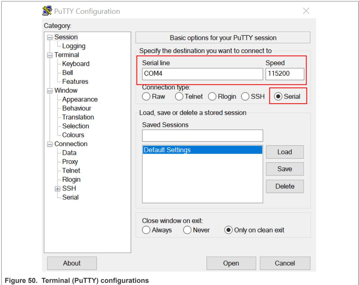
Figure 50. Terminal (PuTTY) configurations
