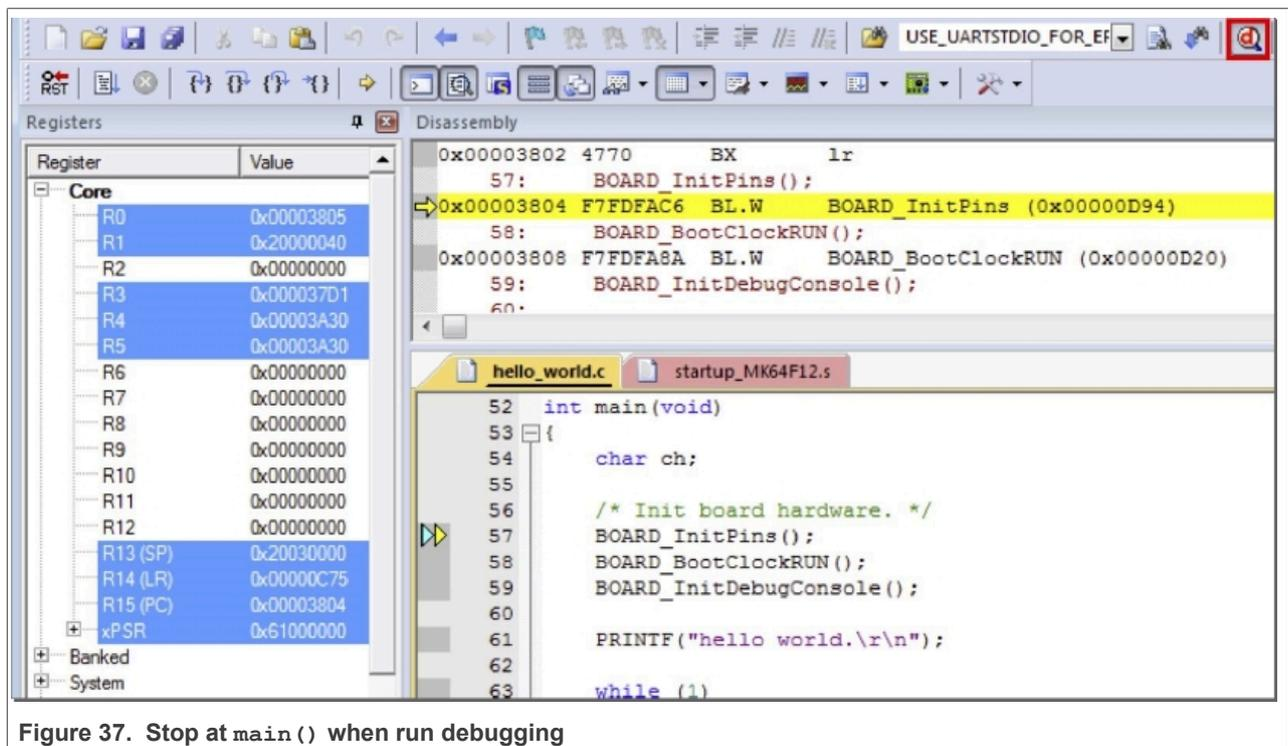
Figure 37. Stop at main() when run debugging
