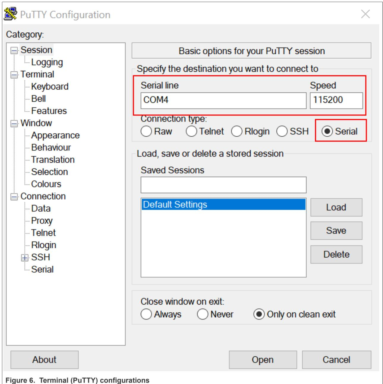
Figure 6. Terminal (PuTTY) configurations
