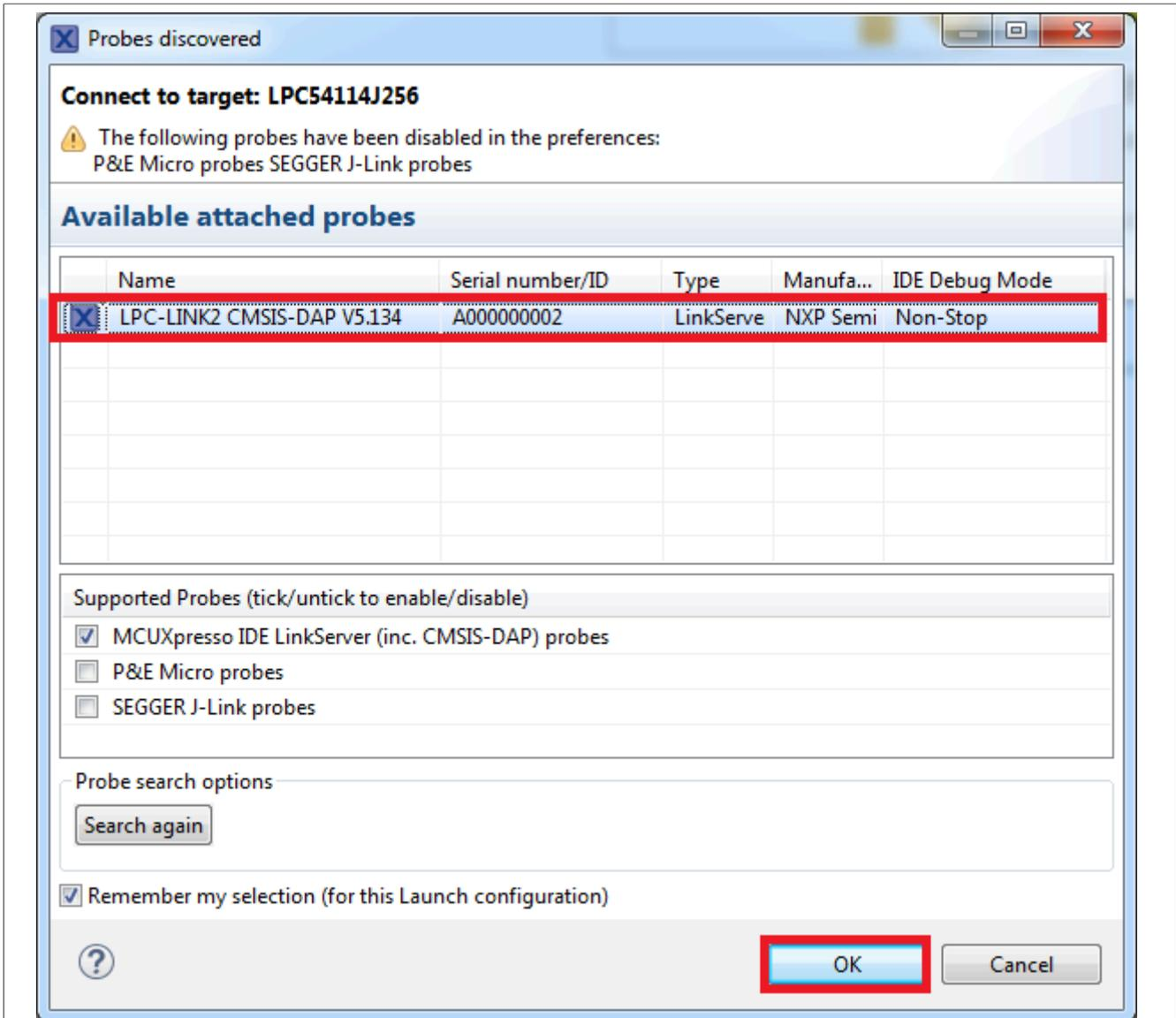
Figure 14. Attached Probes: debug emulator selection
