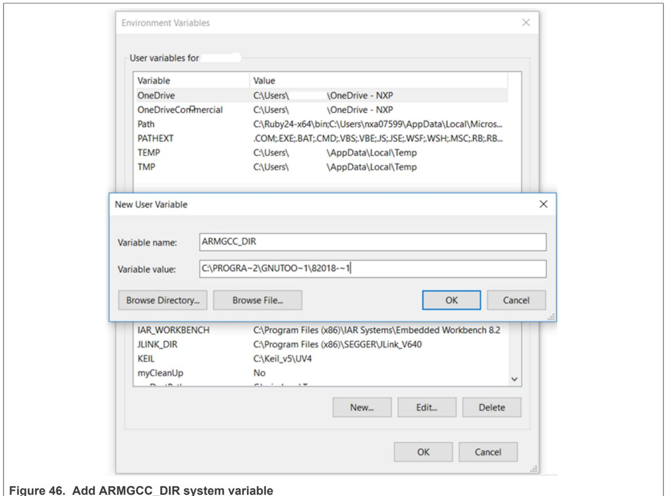
Figure 46. Add ARMGCC\_DIR system variable
