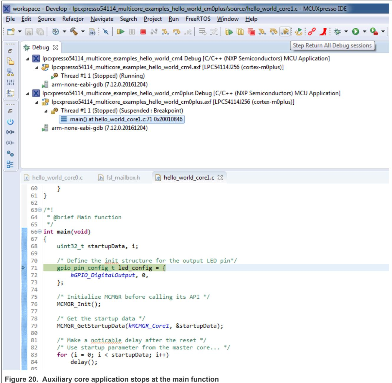
At this point, it is possible to suspend and resume individual cores independently. It is also possible to make synchronous suspension and resumption of both the cores. This is done either by selecting both opened debug sessions (multiple selections) and clicking the “Suspend” / “Resume” control button, or just using the “Suspend All Debug sessions” and the “Resume All Debug sessions” buttons.
