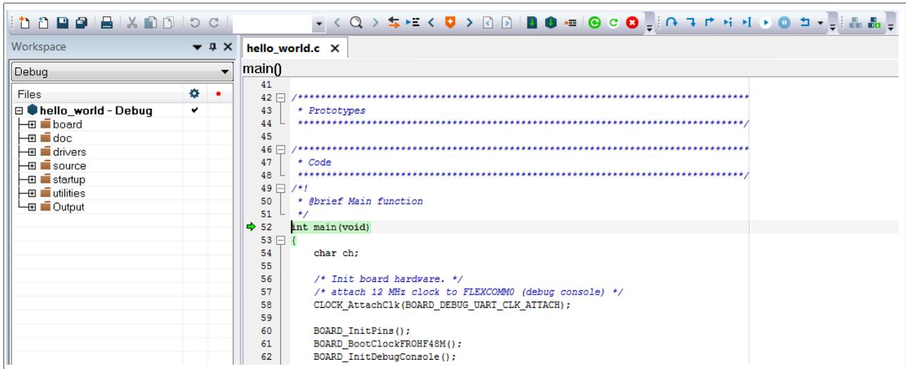
Figure 27. Stop at main() when running debugging
