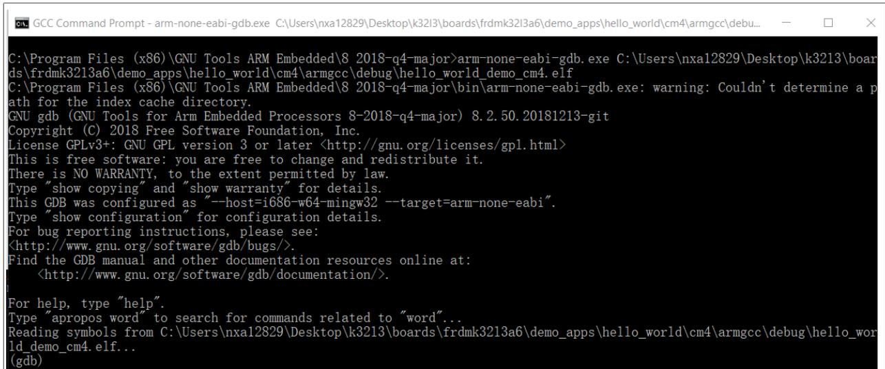
Figure 53. Run arm-none-eabi-gdb
