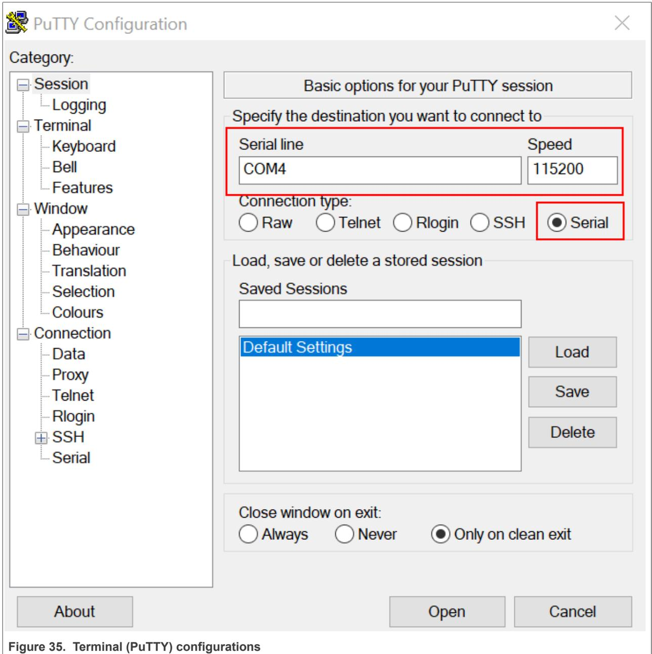
Figure 35. Terminal (PuTTY) configurations
