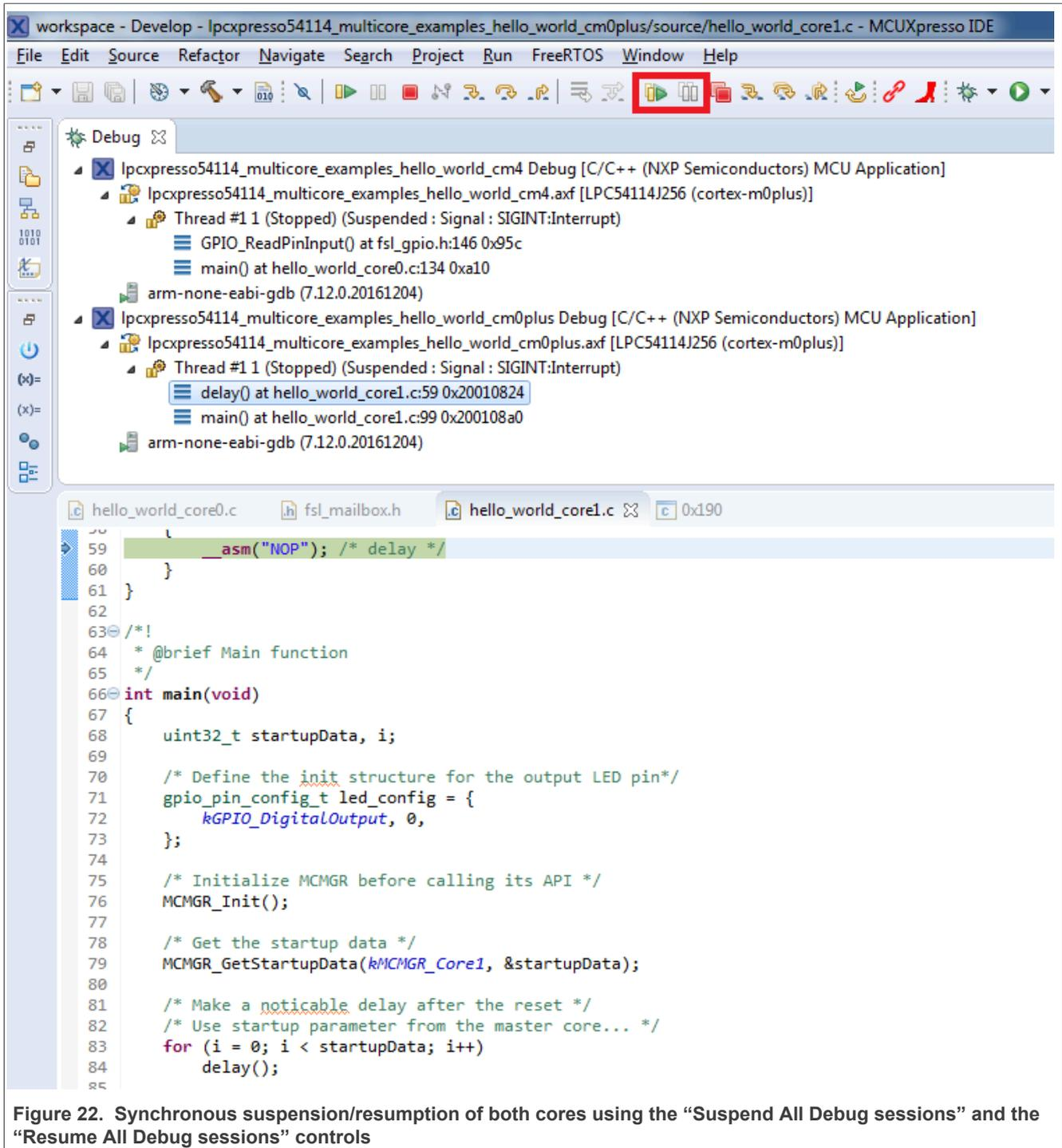
Figure 22. Synchronous suspension/resumption of both cores using the “Suspend All Debug sessions” and the “Resume All Debug sessions” controls
