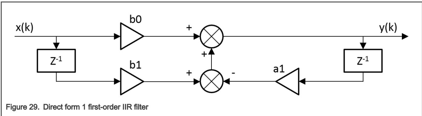
The coefficients of the filter shown in Figure 3-1 can be designed to meet the requirements for the first-order low-pass filter (LPF) or high-pass filter (HPF). The coefficient quantization error is not important in the case of a first-order filter due to a finite precision
