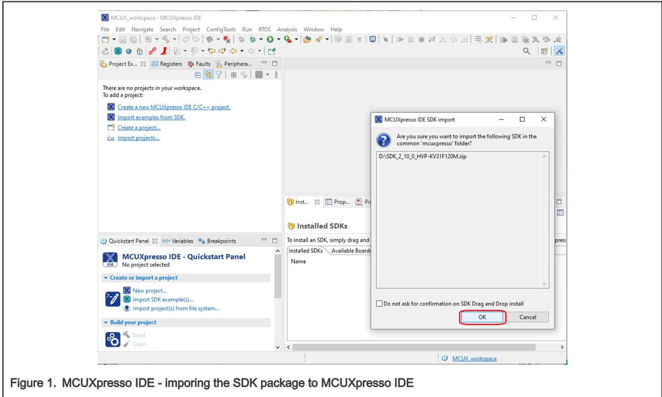
Figure 1. MCUXpresso IDE - importing the SDK package to MCUXpresso IDE
