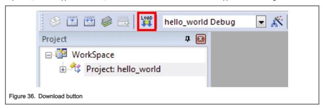
5. After clicking the **Download** button, the application downloads to the target and is running. To debug the application, click the **Start/Stop Debug Session** button, highlighted in red.
