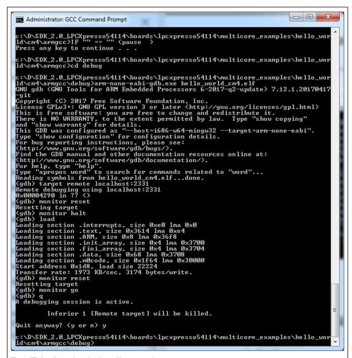
Figure 57. Loading and running the multicore example
