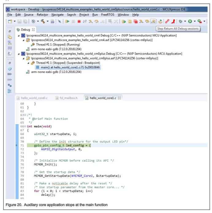
At this point, it is possible to suspend and resume individual cores independently. It is also possible to make synchronous suspension and resumption of both the cores. This is done either by selecting both opened debug sessions (multiple selection) and clicking the "Suspend" / "Resume" control button, or just using the "Suspend All Debug sessions" and the "Resume All Debug sessions" buttons.
