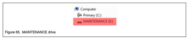
4. Drag and drop the new firmware image onto the MAINTENANCE drive.
