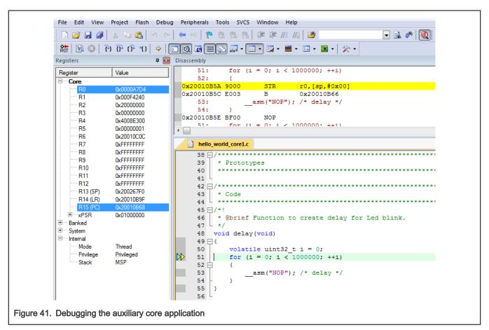
Arm describes multi-core debugging using the NXP LPC54114 Cortex-M4/M0+ dual-core processor and Keil uVision IDE in Application Note 318 at <a href="https://www.keil.com/appnotes/docs/apnt-318.asp">www.keil.com/appnotes/docs/apnt-318.asp</a>. The associated video can be found here.
