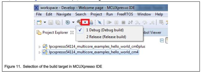
The project starts building after the build target is selected. Because of the project reference settings in multicore projects, triggering the build of the primary core application (cm4) also causes the referenced auxiliary core application (cm0plus) to build.
