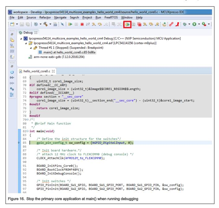
After clicking the "Resume All Debug sessions" button, the hello\_world multicore application runs and a banner is displayed on the terminal. If this is not the case, check your terminal settings and connections.
