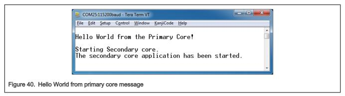
An LED controlled by the auxiliary core starts flashing indicating that the auxiliary core has been released from the reset and is running correctly.
