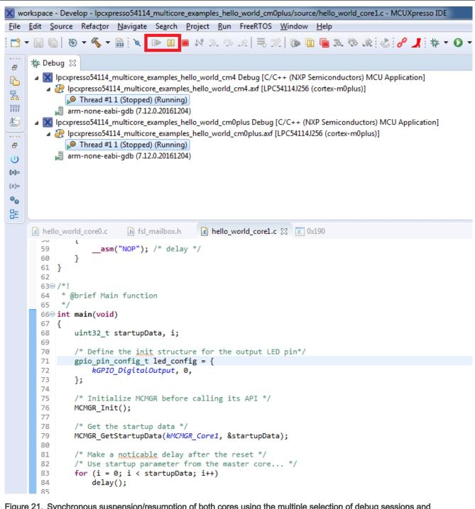
Figure 21. Synchronous suspension/resumption of both cores using the multiple selection of debug sessions and "Suspend"/"Resume" controls
