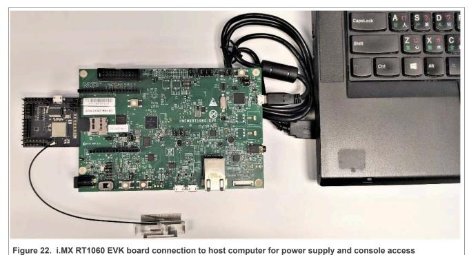
rigure 22. Innex Ki 1999 2 vik board connection to nost compater for power supply and console access
