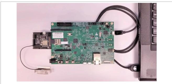
Figure 6. i.MX RT1060 EVK board connection to the host computer for power supply and console access
