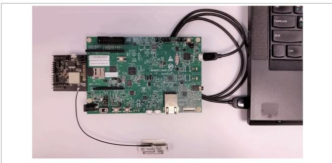
Figure 16. i.MX RT1060 EVK connection to the host computer for power supply and console access
