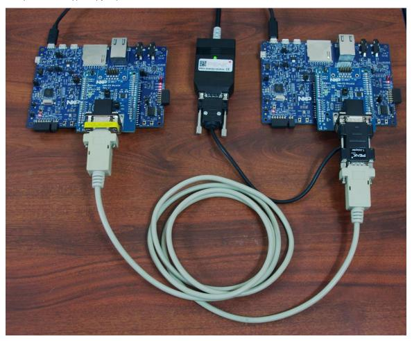
The setup in the previous picture consist of one LPCXpresso54628 and LPCxpresso54S018 each with a CAN shield and termination resistors enabled. A RS232 cable with one gender changer, a 'Y' (or'T') cable and a PCAN-USB FD to monitor the CANopen communication.
