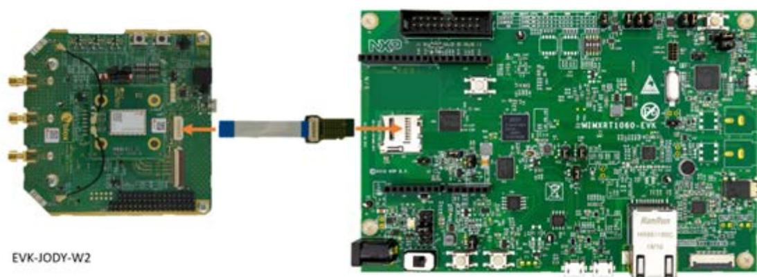
Figure 32. u-blox EVK-JODY-W2 connected to i.MX RT1060 EVK using uSD interface
