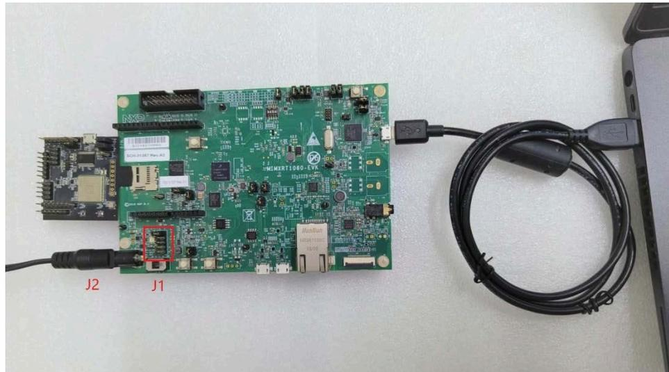
Figure 17. External power supply for i.MX RT1060 EVK board and connection to the host computer for console access
