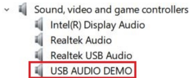
Figure 2: The device enumerated in the device manager
