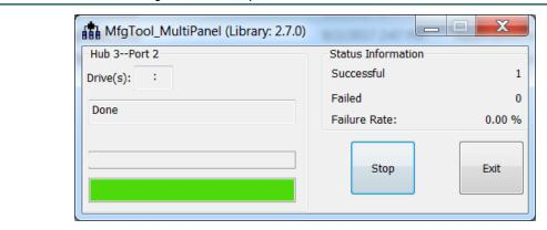
Figure 21. Successful result for programming with MfgTool for Secure Boot
