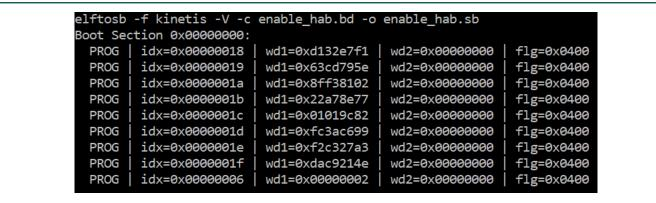
Figure 26. Example command to generate SB file for Fuse programming
