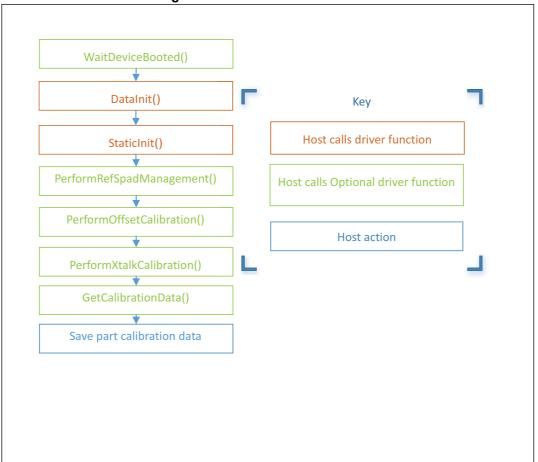
Figure 4. VL53L1X Calibration flow
