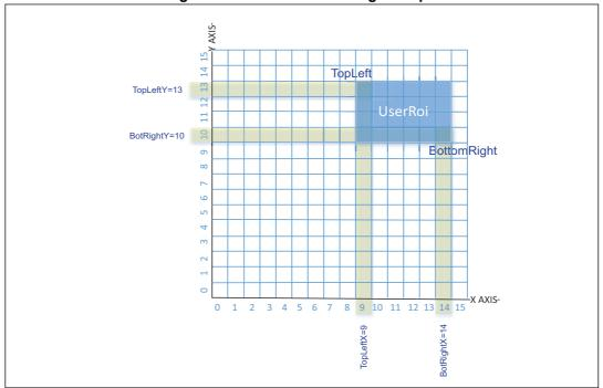
An example of ROI setting is given in Figure 6: VL53L1X ROI setting example
