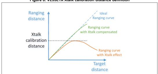
Figure 8. VL53L1X Xtalk calibration distance definition
