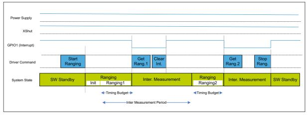
Figure 3. VL53L1X Autonomous Ranging sequence and timings
